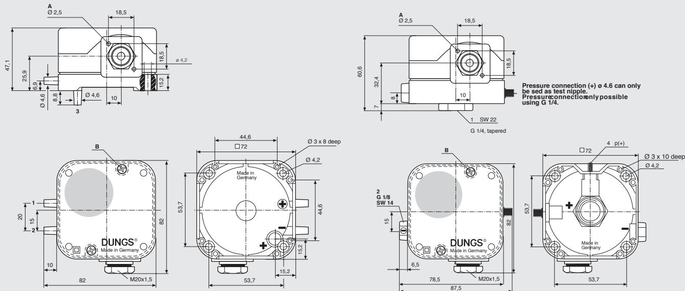
A 2.5 dia for equipment plug as per DIN EN 175 301-803
